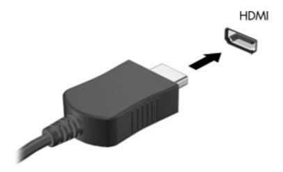
Connect the other end of the cable to the video device, and then refer to the device manufacturer's instructions for additional information. NOTE: For product-specific instructions on switching the screen image, refer to your *Getting Started* guide.
